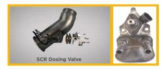
Here are views of the dosing valve found in Pro-MECH's SCR and DEF courses. The two tube connectors on the base of the valve are where coolant is circulated to cool the valve and the upper center port is where the valve releases DEF into the decomposition reactor.
