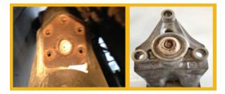
These views show the condition of a dosing valve and its seat on the decomposition reactor after several hundred engine hours on a truck that experienced extensive stop and go driving. The OEM literature indicated that some white residue accumulation is normal. This valve had to be cleaned, and its seat was almost completely clogged.
